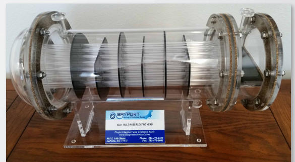
Multi Pass Floating Head Model (115-MPFH)
