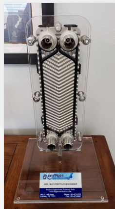
Multi Port Plate Exchanger Model (115-MPPE)
