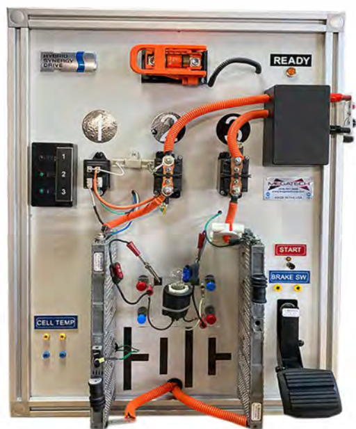
MEG-SMR Hybrid/Electric Vehicle System Main Relay Demonstrator (p. 18)
